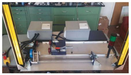
Figure 1. A basic machine like this tape wrapper can be designed to provide the necessary safety using safety relays and light curtain relays.
