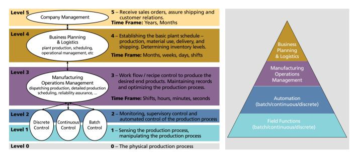
Figure 2. The ISA95 functional model (left) is more traditionally presented as a pyramid.
