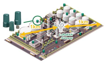
Figure 2. LoRaWAN is well suited to supporting a wide-area network of conditionmonitoring sensors, concentrating all the relevant data in one place.
