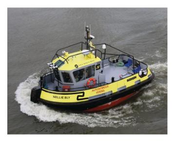
Autonomous operations come to the open ocean with Sea Machines' SM300 system, which uses computer vision and augmented reality. See page 13.
