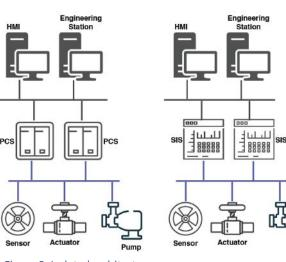
Figure 2. Isolated architecture
