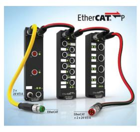
IP67 and IP69K fieldmounted distributed I/O terminals have power and communication in one cable, reducing the amount of cabinet space required on the machine and the number of cables runs back to the controller.
