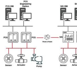
Figure 3. Interfaced architecture
