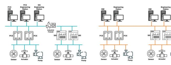
Figure 4. Integrated: restricted architecture
